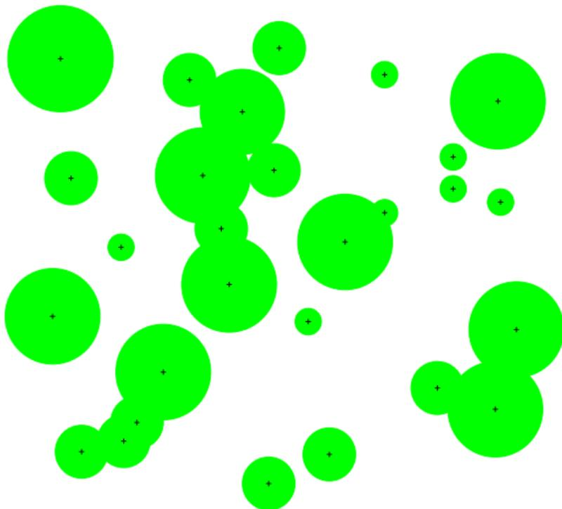
Figure : Green discs representing transmission ranges of transmitters in a wireless network. Picture by B. Błaszczyszyn
